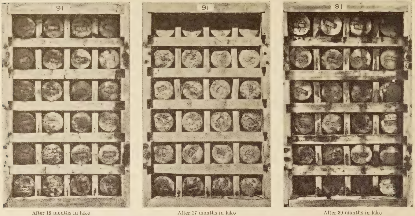
FIGURE 3.—CONDITION OF 1:1½:3 CONCRETE CYLINDERS OF WET CONSISTENCY (BATCH 3, CRATE 91) AFTER 15, 27, AND 39 MONTHS IN MEDICINE LAKE, S. DAK. CURING AND TREATMENT SAME AS IN FIGURE 1
